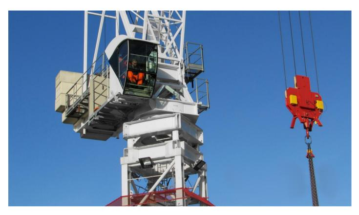
Vantage+ delivers live HD video from crane hook to operator, setting new standards in safety and providing greater operational effectiveness. The ability to remotely stream live and recorded video also allows monitoring by offsite personnel.
